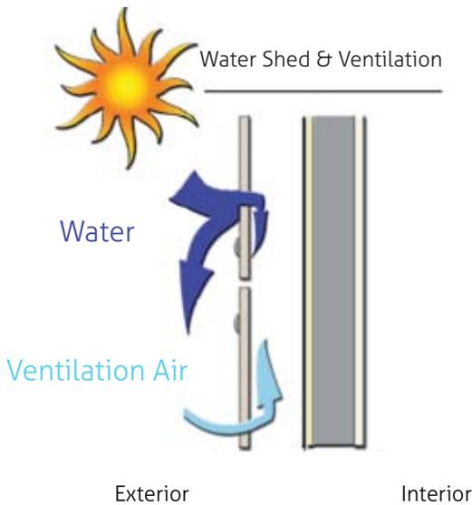
In the summer the ventilated wall is an exceptional reflector of solar radiation. The heat is accumulated on the surface layer & is not passed onto the underlying layers. The heat then escapes the wall thanks to the free-flowing air (The Fireplace Effect).
