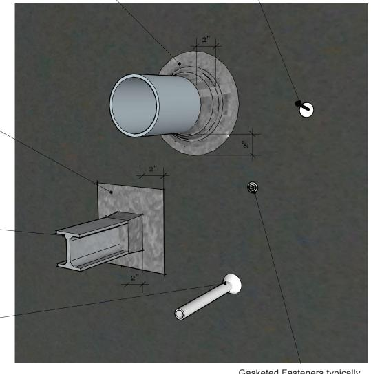
Gasketed Fasteners typically require no additional sealing
